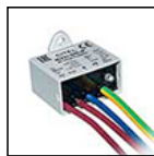
S.2498 SURGE PROTECTION DEVICE 10kV CLASS I Compatible with all lighting fixtures classified under electrical Protection Class I Rated voltage 230-277V SPD type 2+3 Max Surge Protection 10kV IP67
