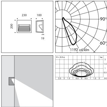
\*Photometric measured using WHITE LED 3000K
