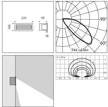
\*Photometric measured using WHITE LED 3000K
