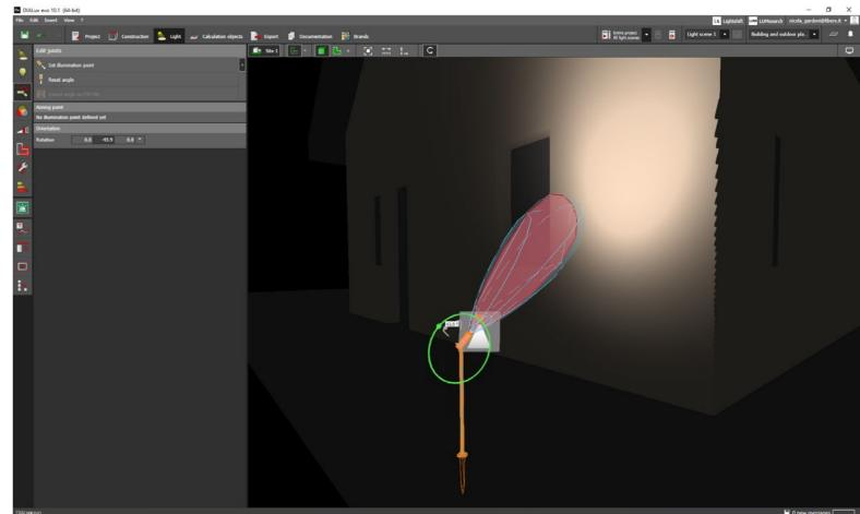
Luminaires with rotable joints can be used on the scene aiming the light photometric emission on the required point.
