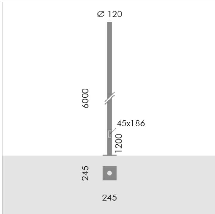
**S.2848****H 6,0m Ø120mm CYLINDRICAL POLE WITH BASE**
