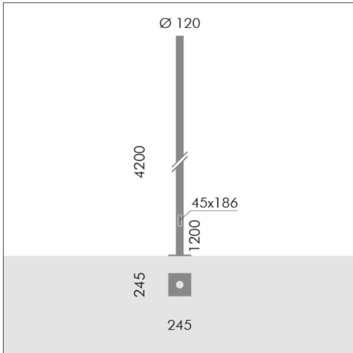
**S.2846****ZYLINDRISCHER MAST H 4,2m Ø120mm MIT
