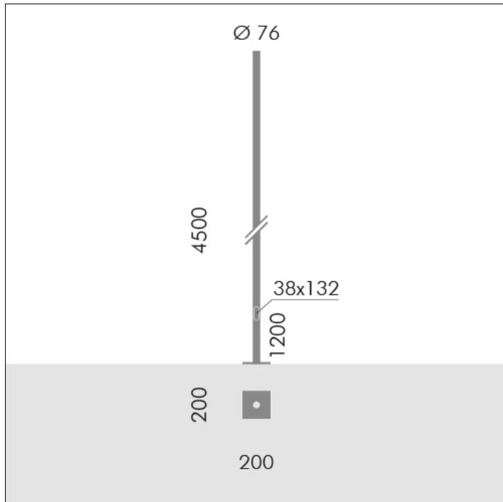
**S.2845****H 4,5m Ø76mm CYLINDRICAL POLE WITH BASE**
