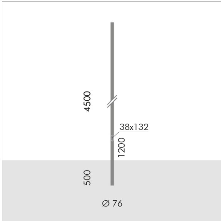
**S.2844****ZYLINDRISCHER MAST H 4,5m Ø76mm MIT ERDSTÜCK**
