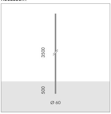
S.2842 H 3,5m Ø60mm CYLINDRICAL POLE TO BE BURIED
