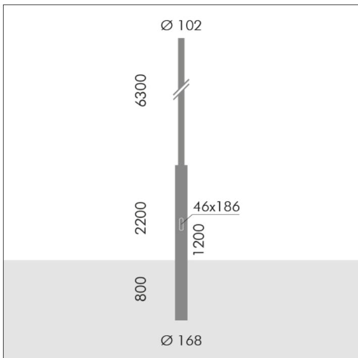
**S.2817****ZYLINDRISCHER MAST H 8,5m D 168mm- D102mm,
