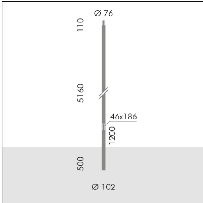
**S.2816****H 5,16m Ø102mm CYLINDRICAL POLE TO BE BURIED
