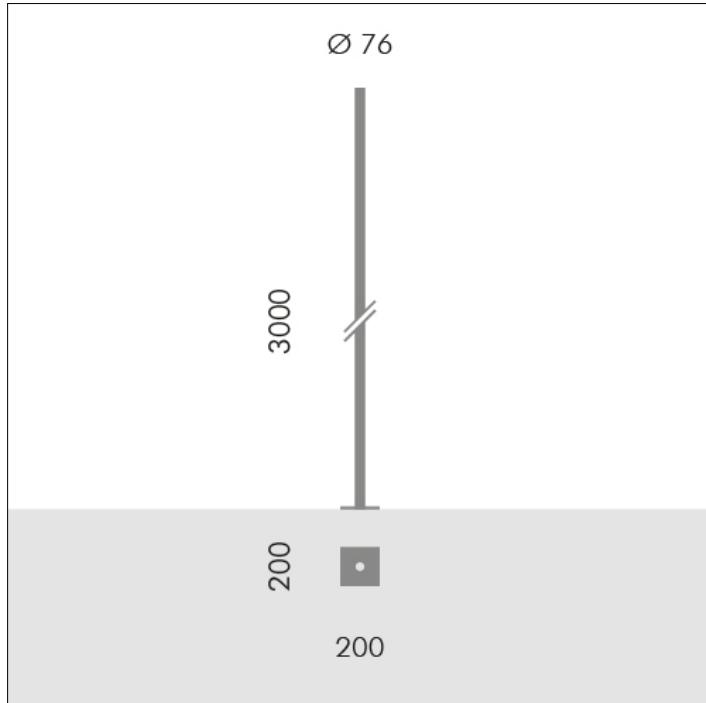
**S.2813****H 3,0m Ø76mm CYLINDRICAL POLE WITH BASE**
