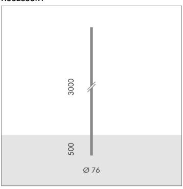
S.2812 H 3,0m Ø76mm CYLINDRICAL POLE TO BE BURIED
