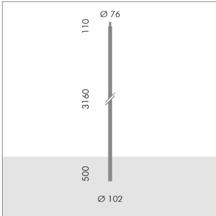
**S.2810****H 3,16m Ø102mm CYLINDRICAL POLE TO BE BURIED
