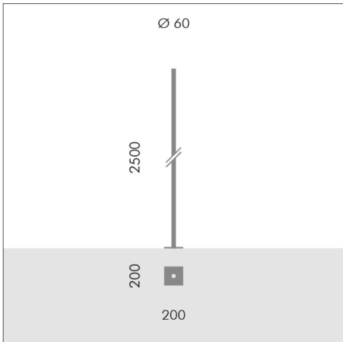
**S.2801****ZYLINDRISCHER MAST H 2,5m Ø60mm MIT
