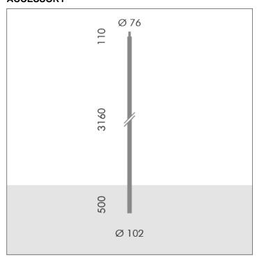
S.2810 H 3,16m Ø102mm CYLINDRICAL POLE TO BE BURIED with Ø76mm SPIGOT
